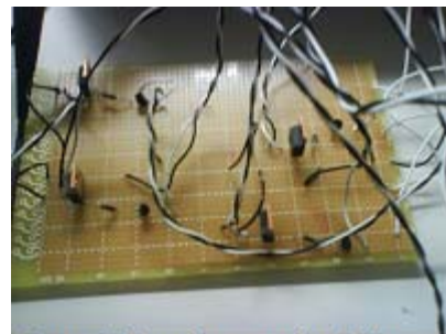
Figure 24, a photograph of the circuit. There are 4 circuits here all working from the same input. White wires are positive, black wires are negative
