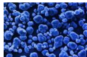
Figure 43: Polyamide seeding particles (PSP) used in the trapping experiment.
